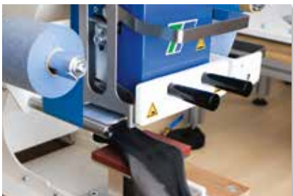
Printing with heat-seal special colour ribbon
