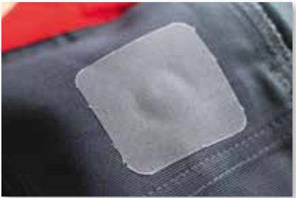
HF transponder with patch material (PA)
