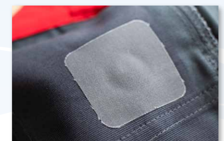
HF transponder with heat-seal material (PA)
