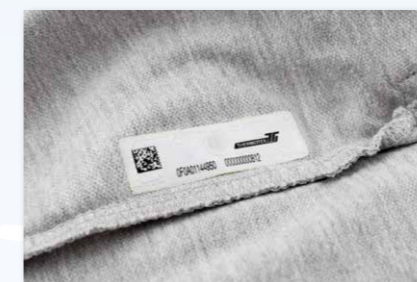
Hired vocational clothing with F10 transponder: inside on the side
