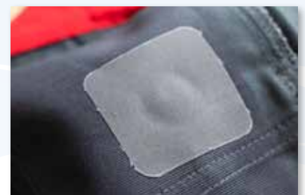
HF tag with heat-seal material (PA)
